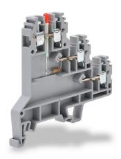
Konnect-It screw triple-level sensor terminal block, connected between levels and power indicator, accepts wire size 24-12 AWG, gray, 24A, PNP LED indicator(s), 35mm DIN rail mount, 100kA SCCR. Package of 20.
