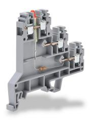
Konnect-It screw triple-level sensor terminal block, connected between levels and power indicator, accepts wire size 24-12 AWG, gray, 24A, NPN LED indicator(s), 35mm DIN rail mount, 100kA SCCR. Package of 20.
