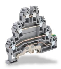
Konnect-It screw triple-level feedthrough terminal block, with ground, accepts wire size 24-12 AWG, gray, 24A, 35mm DIN rail mount, 100kA SCCR. Package of 20. For use with jumpers KN-2JTL12, KN-3JTL12, KN-4JTL12 and KN-10JTL12.
