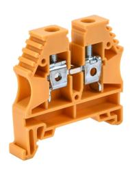
Konnect-It screw single-level feedthrough terminal block, accepts wire size 26-8 AWG, yellow, 50A, 35mm DIN rail mount, 100kA SCCR. Package of 60. For use with jumpers KN-2J8, KN-3J8, KN-4J8 and KN-10J8.
