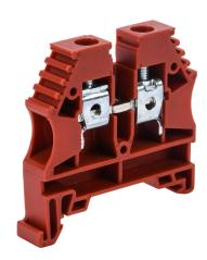
Konnect-It screw single-level feedthrough terminal block, accepts wire size 26-8 AWG, red, 50A, 35mm DIN rail mount, 100kA SCCR. Package of 20. For use with jumpers KN-2J8, KN-3J8, KN-4J8 and KN-10J8.
