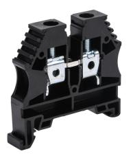
Konnect-It screw single-level feedthrough terminal block, accepts wire size 26-8 AWG, black, 50A, 35mm DIN rail mount, 100kA SCCR. Package of 60. For use with jumpers KN-2J8, KN-3J8, KN-4J8 and KN-10J8.
