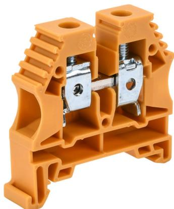
Konnect-It screw single-level feedthrough terminal block, accepts wire size 16-6 AWG, yellow, 65A, 35mm DIN rail mount, 100kA SCCR. Package of 50. For use with jumpers KN-2J6, KN-3J6, KN-4J6 and KN-10J6.
