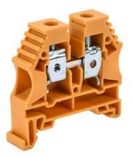
Konnect-It screw single-level feedthrough terminal block, accepts wire size 16-6 AWG, yellow, 65A, 35mm DIN rail mount, 100kA SCCR. Package of 50. For use with jumpers KN-2J6, KN-3J6, KN-4J6 and KN-10J6.
