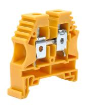
Konnect-It screw single-level feedthrough terminal block, accepts wire size 16-6 AWG, yellow, 65A, 35mm DIN rail mount, 100kA SCCR. Package of 25. For use with jumpers KN-2J6, KN-3J6, KN-4J6 and KN-10J6.
