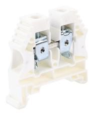
Konnect-It screw single-level feedthrough terminal block, accepts wire size 16-6 AWG, white, 65A, 35mm DIN rail mount, 100kA SCCR. Package of 50. For use with jumpers KN-2J6, KN-3J6, KN-4J6 and KN-10J6.
