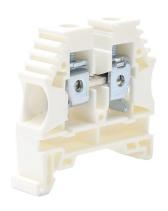
Konnect-It screw single-level feedthrough terminal block, accepts wire size 16-6 AWG, white, 65A, 35mm DIN rail mount, 100kA SCCR. Package of 25. For use with jumpers KN-2J6, KN-3J6, KN-4J6 and KN-10J6.
