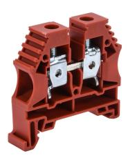
Konnect-It screw single-level feedthrough terminal block, accepts wire size 16-6 AWG, red, 65A, 35mm DIN rail mount, 100kA SCCR. Package of 50. For use with jumpers KN-2J6, KN-3J6, KN-4J6 and KN-10J6.
