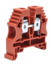
Konnect-It screw single-level feedthrough terminal block, accepts wire size 16-6 AWG, red, 65A, 35mm DIN rail mount, 100kA SCCR. Package of 25. For use with jumpers KN-2J6, KN-3J6, KN-4J6 and KN-10J6.
