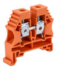
Konnect-It screw single-level feedthrough terminal block, accepts wire size 16-6 AWG, orange, 65A, 35mm DIN rail mount, 100kA SCCR. Package of 50. For use with jumpers KN-2J6, KN-3J6, KN-4J6 and KN-10J6.
