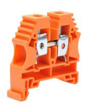
Konnect-It screw single-level feedthrough terminal block, accepts wire size 16-6 AWG, orange, 65A, 35mm DIN rail mount, 100kA SCCR. Package of 25. For use with jumpers KN-2J6, KN-3J6, KN-4J6 and KN-10J6.
