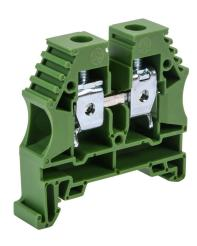
Konnect-It screw single-level feedthrough terminal block, accepts wire size 16-6 AWG, green, 65A, 35mm DIN rail mount, 100kA SCCR. Package of 50. For use with jumpers KN-2J6, KN-3J6, KN-4J6 and KN-10J6.
