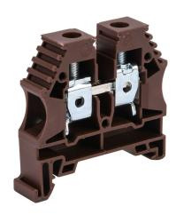
Konnect-It screw single-level feedthrough terminal block, accepts wire size 16-6 AWG, brown, 65A, 35mm DIN rail mount, 100kA SCCR. Package of 50. For use with jumpers KN-2J6, KN-3J6, KN-4J6 and KN-10J6.
