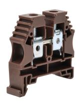
Konnect-It screw single-level feedthrough terminal block, accepts wire size 16-6 AWG, brown, 65A, 35mm DIN rail mount, 100kA SCCR. Package of 25. For use with jumpers KN-2J6, KN-3J6, KN-4J6 and KN-10J6.
