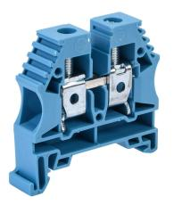
Konnect-It screw single-level feedthrough terminal block, accepts wire size 16-6 AWG, blue, 65A, 35mm DIN rail mount, 100kA SCCR. Package of 50. For use with jumpers KN-2J6, KN-3J6, KN-4J6 and KN-10J6.
