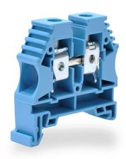
Konnect-It screw single-level feedthrough terminal block, accepts wire size 16-6 AWG, blue, 65A, 35mm DIN rail mount, 100kA SCCR. Package of 25. For use with jumpers KN-2J6, KN-3J6, KN-4J6 or KN-10J6.
