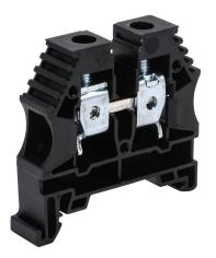
Konnect-It screw single-level feedthrough terminal block, accepts wire size 16-6 AWG, black, 65A, 35mm DIN rail mount, 100kA SCCR. Package of 50. For use with jumpers KN-2J6, KN-3J6, KN-4J6 and KN-10J6.
