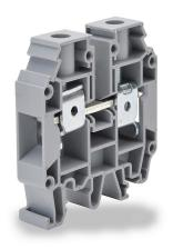
Konnect-It screw single-level feedthrough terminal block, accepts wire size 12-4 AWG, gray, 80A, 35mm DIN rail mount, 100kA SCCR. Package of 50. For use with jumpers KN-2J4, KN-3J4, KN-4J4 and KN-10J4.
