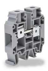
Konnect-It screw single-level feedthrough terminal block, accepts wire size 12-4 AWG, gray, 80A, 35mm DIN rail mount, 100kA SCCR. Package of 50. For use with jumpers KN-2J4, KN-3J4, KN-4J4 and KN-10J4.
