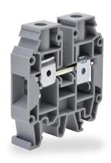
Konnect-It screw single-level feedthrough terminal block, accepts wire size 12-4 AWG, gray, 80A, 35mm DIN rail mount, 100kA SCCR. Package of 25. For use with jumpers KN-2J4, KN-3J4, KN-4J4 or KN-10J4.
