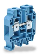
Konnect-It screw single-level feedthrough terminal block, accepts wire size 12-4 AWG, blue, 80A, 35mm DIN rail mount, 100kA SCCR. Package of 50. For use with jumpers KN-2J4, KN-3J4, KN-4J4 and KN-10J4.
