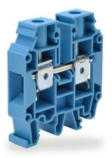
Konnect-It screw single-level feedthrough terminal block, accepts wire size 12-4 AWG, blue, 80A, 35mm DIN rail mount, 100kA SCCR. Package of 25. For use with jumpers KN-2J4, KN-3J4, KN-4J4 or KN-10J4.
