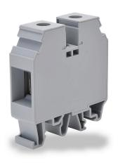
Konnect-It screw single-level feedthrough terminal block, accepts wire size 12-2 AWG, gray, 115A, 35mm DIN rail mount, 100kA SCCR. Package of 40. For use with jumpers KN-2J2, KN-3J2, KN-4J2 and KN-10J2.
