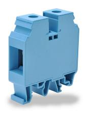
Konnect-It screw single-level feedthrough terminal block, accepts wire size 12-2 AWG, blue, 115A, 35mm DIN rail mount, 100kA SCCR. Package of 40. For use with jumpers KN-2J2, KN-3J2, KN-4J2 and KN-10J2.
