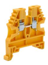
Konnect-It screw single-level feedthrough terminal block, accepts wire size 26-12 AWG, yellow, 20A, 35mm DIN rail mount, 100kA SCCR. Package of 25. For use with jumpers KN-2J12, KN-3J12, KN-4J12 and KN-10J12.
