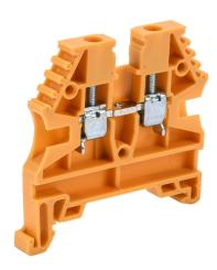
Konnect-It screw single-level feedthrough terminal block, accepts wire size 26-12 AWG, yellow, 20A, 35mm DIN rail mount, 100kA SCCR. Package of 100. For use with jumpers KN-2J12, KN-3J12, KN-4J12 and KN-10J12.
