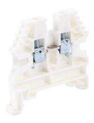
Konnect-It screw single-level feedthrough terminal block, accepts wire size 26-12 AWG, white, 20A, 35mm DIN rail mount, 100kA SCCR. Package of 100. For use with jumpers KN-2J12, KN-3J12, KN-4J12 and KN-10J12.
