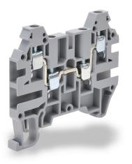
Konnect-It screw common point single-level feedthrough terminal block, two-connection to two-connection, accepts wire size 26-12 AWG, gray, 20A, 35mm DIN rail mount, 100kA SCCR. Package of 100. For use with jumpers KN-2JM12, KN-3JM12, KN-4JM12 and KN-10JM12.
