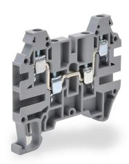
Konnect-It screw common point single-level feedthrough terminal block, two-connection to two-connection, accepts wire size 26-12 AWG, gray, 20A, 35mm DIN rail mount, 100kA SCCR. Package of 25. For use with jumpers KN-2JM12, KN-3JM12, KN-4JM12 and KN-10JM12.
