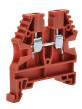
Konnect-It screw single-level feedthrough terminal block, accepts wire size 26-12 AWG, red, 20A, 35mm DIN rail mount, 100kA SCCR. Package of 25. For use with jumpers KN-2J12, KN-3J12, KN-4J12 and KN-10J12.
