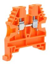
Konnect-It screw single-level feedthrough terminal block, accepts wire size 26-12 AWG, orange, 20A, 35mm DIN rail mount, 100kA SCCR. Package of 25. For use with jumpers KN-2J12, KN-3J12, KN-4J12 and KN-10J12.
