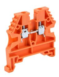
Konnect-It screw single-level feedthrough terminal block, accepts wire size 26-12 AWG, orange, 20A, 35mm DIN rail mount, 100kA SCCR. Package of 100. For use with jumpers KN-2J12, KN-3J12, KN-4J12 and KN-10J12.
