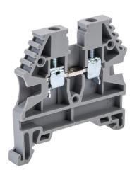
Konnect-It screw single-level feedthrough terminal block, accepts wire size 26-12 AWG, gray, 20A, 35mm DIN rail mount, 100kA SCCR. Package of 100. For use with jumpers KN-2J12, KN-3J12, KN-4J12 and KN-10J12.
