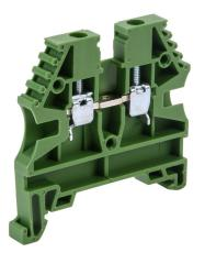
Konnect-It screw single-level feedthrough terminal block, accepts wire size 26-12 AWG, green, 20A, 35mm DIN rail mount, 100kA SCCR. Package of 100. For use with jumpers KN-2J12, KN-3J12, KN-4J12 and KN-10J12.
