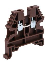
Konnect-It screw single-level feedthrough terminal block, accepts wire size 26-12 AWG, brown, 20A, 35mm DIN rail mount, 100kA SCCR. Package of 100. For use with jumpers KN-2J12, KN-3J12, KN-4J12 and KN-10J12.
