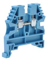
Konnect-It screw single-level feedthrough terminal block, accepts wire size 26-12 AWG, blue, 20A, 35mm DIN rail mount, 100kA SCCR. Package of 25. For use with jumpers KN-2J12, KN-3J12, KN-4J12 and KN-10J12.
