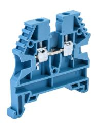
Konnect-It screw single-level feedthrough terminal block, accepts wire size 26-12 AWG, blue, 20A, 35mm DIN rail mount, 100kA SCCR. Package of 100. For use with jumpers KN-2J12, KN-3J12, KN-4J12 and KN-10J12.
