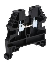
Konnect-It screw single-level feedthrough terminal block, accepts wire size 26-12 AWG, black, 20A, 35mm DIN rail mount, 100kA SCCR. Package of 100. For use with jumpers KN-2J12, KN-3J12, KN-4J12 and KN-10J12.
