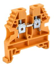
Konnect-It screw single-level feedthrough terminal block, accepts wire size 26-10 AWG, yellow, 30A, 35mm DIN rail mount, 100kA SCCR. Package of 80. For use with jumpers KN-2J10, KN-3J10, KN-4J10 and KN-10J10.
