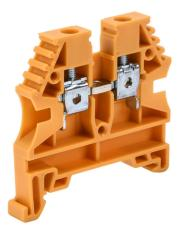
Konnect-It screw single-level feedthrough terminal block, accepts wire size 26-10 AWG, yellow, 30A, 35mm DIN rail mount, 100kA SCCR. Package of 20. For use with jumpers KN-2J10, KN-3J10, KN-4J10 and KN-10J10.
