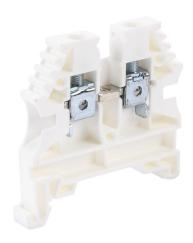
Konnect-It screw single-level feedthrough terminal block, accepts wire size 26-10 AWG, white, 30A, 35mm DIN rail mount, 100kA SCCR. Package of 80. For use with jumpers KN-2J10, KN-3J10, KN-4J10 and KN-10J10.
