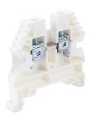
Konnect-It screw single-level feedthrough terminal block, accepts wire size 26-10 AWG, white, 30A, 35mm DIN rail mount, 100kA SCCR. Package of 20. For use with jumpers KN-2J10, KN-3J10, KN-4J10 and KN-10J10.
