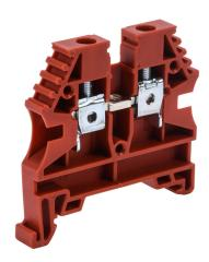
Konnect-It screw single-level feedthrough terminal block, accepts wire size 26-10 AWG, red, 30A, 35mm DIN rail mount, 100kA SCCR. Package of 20. For use with jumpers KN-2J10, KN-3J10, KN-4J10 and KN-10J10.
