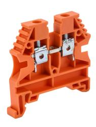
Konnect-It screw single-level feedthrough terminal block, accepts wire size 26-10 AWG, orange, 30A, 35mm DIN rail mount, 100kA SCCR. Package of 20. For use with jumpers KN-2J10, KN-3J10, KN-4J10 and KN-10J10.
