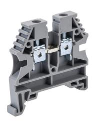
Konnect-It screw single-level feedthrough terminal block, accepts wire size 26-10 AWG, gray, 30A, 35mm DIN rail mount, 100kA SCCR. Package of 80. For use with jumpers KN-2J10, KN-3J10, KN-4J10 and KN-10J10.
