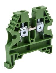
Konnect-It screw single-level feedthrough terminal block, accepts wire size 26-10 AWG, green, 30A, 35mm DIN rail mount, 100kA SCCR. Package of 80. For use with jumpers KN-2J10, KN-3J10, KN-4J10 and KN-10J10.
