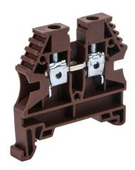
Konnect-It screw single-level feedthrough terminal block, accepts wire size 26-10 AWG, brown, 30A, 35mm DIN rail mount, 100kA SCCR. Package of 80. For use with jumpers KN-2J10, KN-3J10, KN-4J10 and KN-10J10.
