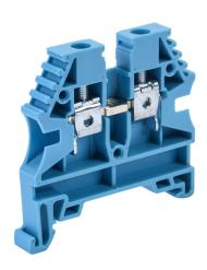
Konnect-It screw single-level feedthrough terminal block, accepts wire size 26-10 AWG, blue, 30A, 35mm DIN rail mount, 100kA SCCR. Package of 80. For use with jumpers KN-2J10, KN-3J10, KN-4J10 and KN-10J10.
